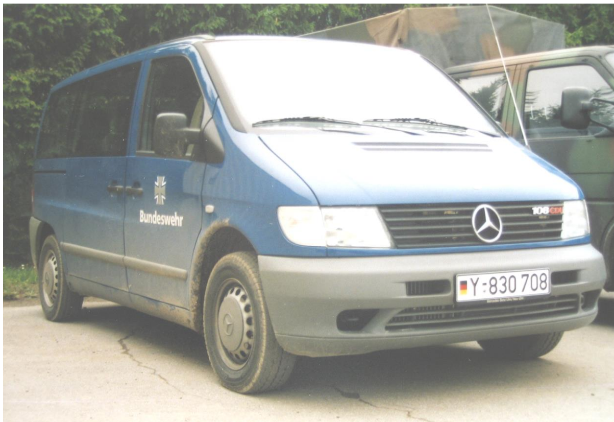
Mercedes-Benz Vito 108 CDI. With a GVW of 2,700 kg the payload can be up to 800 kg.
