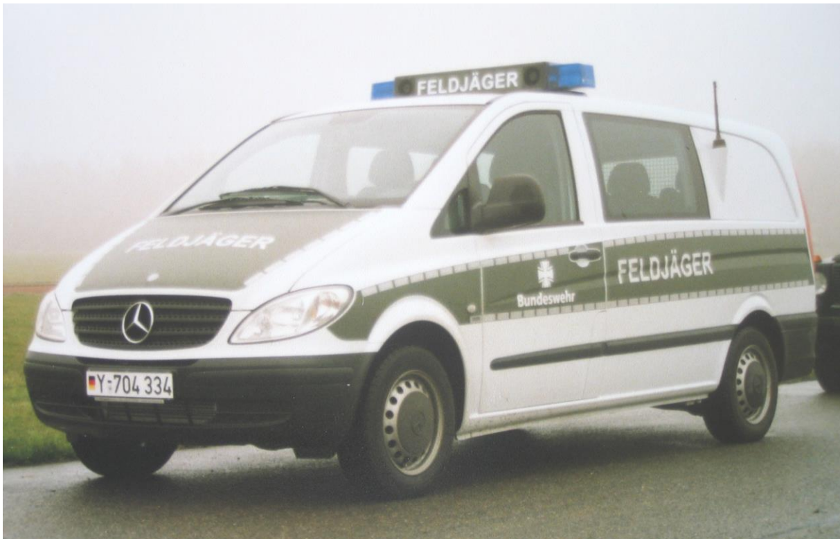
Mercedes-Benz DC Vito (4x2) 111 CDI Feldjäger (Military Police) with 3,200 mm wheelbase. The 4-cylinder engine develops 80 kW (109 hp). Displacement is 2,148 ccm. All markings are fitted on as foils and can be removed easily to sell the vehicle on the private market after a defined amount of kilometres has been reached.
