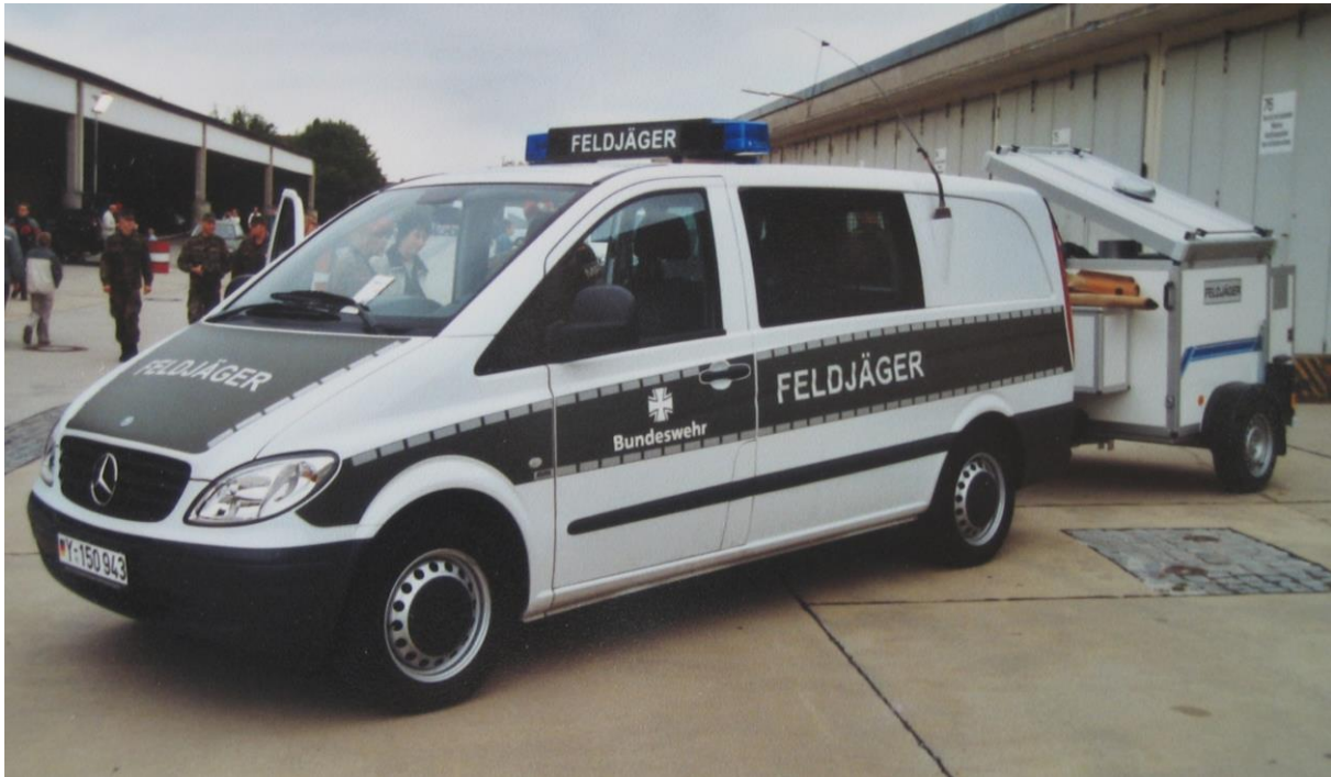
Mercedes-Benz DC Vito (4x2) 115 CDI Feldjäger (Military Police). The 4-cylinder engine develops 110 kW (150 hp) at 1,800 to 2,400 rpm. Maximum speed is 180 km/h on roads with canine systems trailer type Bamberg with two boxes for the transport of dogs. Empty weight is 2,380 kg.
