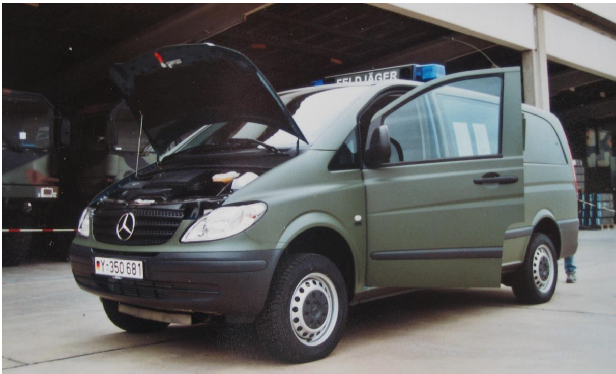
Mercedes-Benz DC Vito (4x4) 115 CDI Feldjäger (Military Police). This vehicle with a wheelbase of 3,200 mm is not naturally olive and the military look can be removed easily. The 4-cylinder engine develops 110 kW (150 hp) at 1,800 to 2,400 rpm. Displacement is 2,148 cc. Empty weight is 2,380 kg. Special equipment includes: double-flash special emergency-light type DBS 2000/3000 (12/24 V), horn, antenna mount, information panel at the rear to stop vehicles for inspection, microphone and outboard loudspeaker installation, Mag-Lite flash-lights for driver and co-driver, telephone installation for hands-off communication, air conditioning, heater, rifle racks for G-36 assault rifles, and radio system FuG SEM 80.
