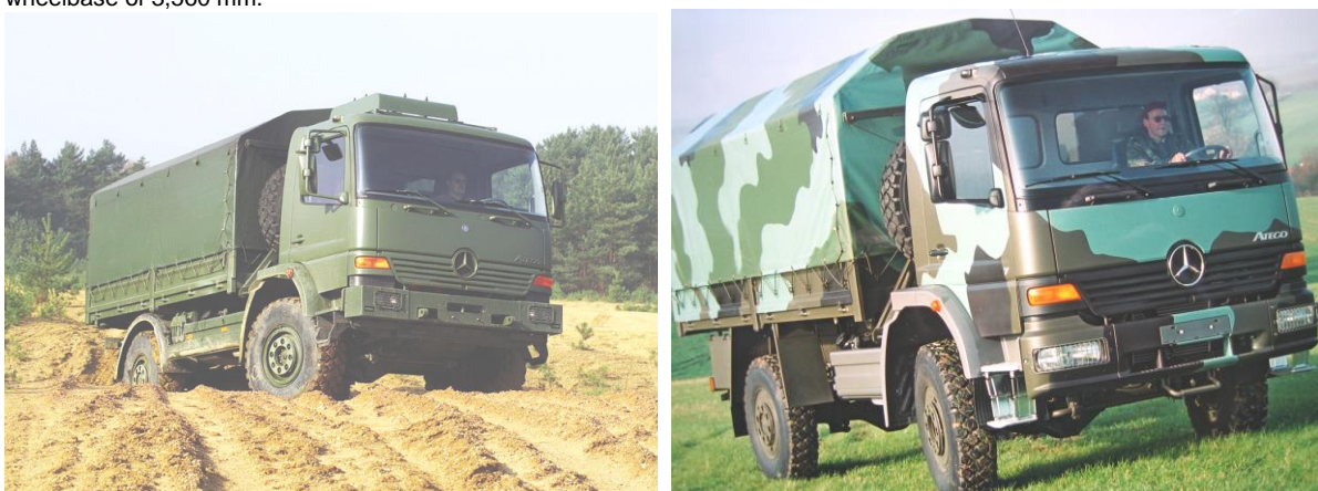
Left: Mercedes-Benz Atego 1323 A, the tactical variant with protected front lights and the capability to fit a ring-mount for a GPMG. Right: Mercedes-Benz Atego 1323 A with single tyres showing a three-tone camouflage pattern for an export customer.
