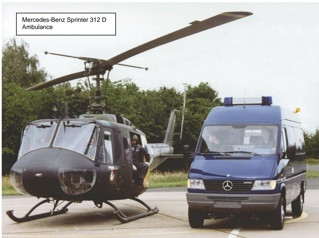
The New Sprinter is essentially a civilian (4x2) van modified by the fitting of an all-wheel drive system. After activating the (4x4) mode the torque moment is distributed 50 : 50 between front and rear axles.
